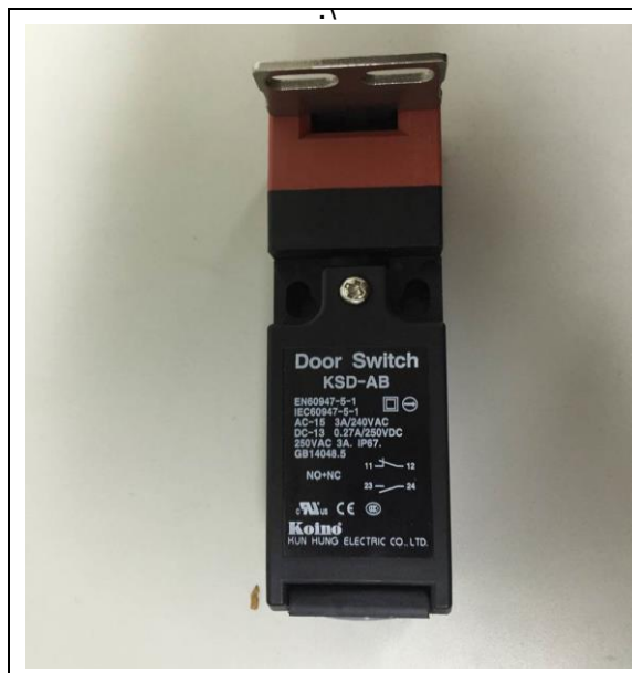
[Photo 1. Safety Door Switch]
